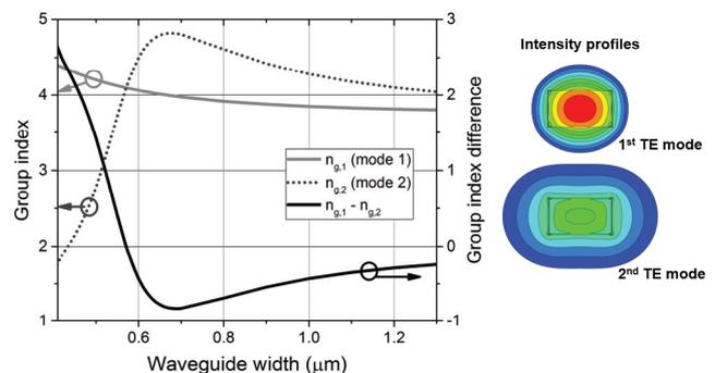
Fig. 2. Group index versus waveguide width of the first and second order TE modes for a DMW and the resulting group index difference are shown at  $\lambda = 1550$  nm, simulated using the FIMMWAVE film mode matching solver. The silicon layer has a thickness of 250 nm. Exemplary mode intensity profiles are also shown on the right for a waveguide width of 420 nm.
