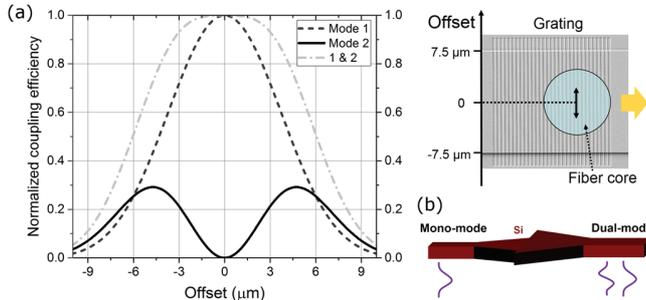
Fig. 3. (a) Approximated coupling efficiency to the first and second order TE modes for a 15  $\mu\text{m}$  broad SOI grating coupler versus lateral offset of the fiber core with respect to the grating coupler center. The Gaussian fiber mode profile has a mode field diameter of 10.4  $\mu\text{m}$ . (b) Suggestion for dual-mode excitation with mono-mode waveguide input enabled by two laterally displaced tapers.
