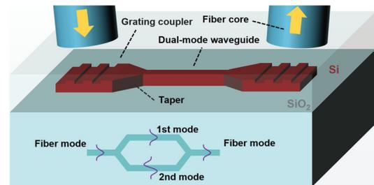
Fig. 1. Schematic design of a dual-mode waveguide interferometer. The signal of a single mode fiber excites different modes in a grating coupler. The excited modes are tapered. Only the two lowest order modes can propagate further in the dual-mode waveguide. Subsequently, the modes travel through the waveguide and are combined by the outcoupling process. Coupling efficiency depends on the phase difference between the modes.
