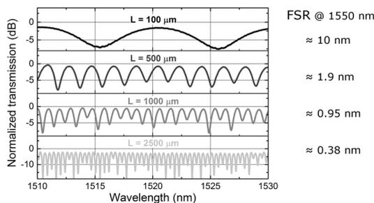
Fig. 4. Optical transmission of different DMWs with grating coupler input and output versus wavelength normalized to the zero-offset transmission. The presented FSR values are calculated for different spectral maxima and minima in the vicinity of 1550 nm. The used TE grating couplers have a 400  $\mu\text{m}$  long taper.
