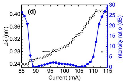
Fig. 3. (a) Lasing spectra at the injection current of 90 mA, and (b) wavelength interval and intensity ratio of the dual-wavelength versus the injection current.
