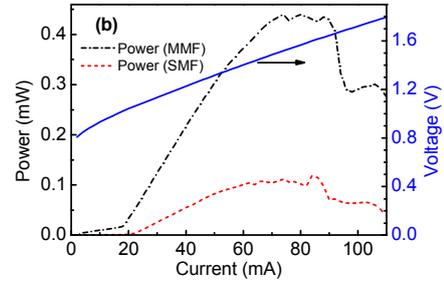
Fig. 2. (a) Microscopic image of the fabricated square microlaser. (b) Output powers coupled into MMF (dash dot line) and SMF (dash line), and the applied voltage (solid line) versus the continuous-wave injection current.
