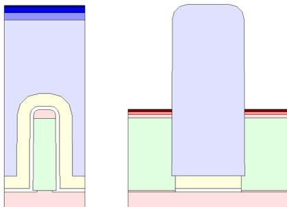
Figure 2. Cross section showing the Fin (left) and the Gate (right) with their curvatures, which are the parameters in the reduced basis study.
