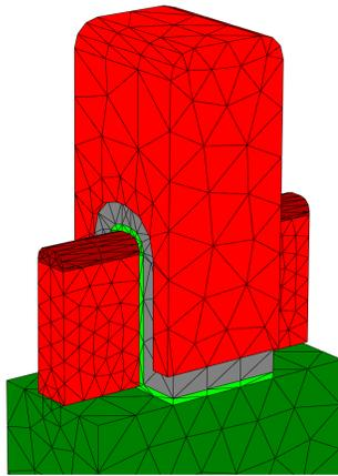
Figure 1. Part of a FinFET, meshed with tetrahedrons, displaying the Fin and the Gate structure. All geometric quantities like widths, heights, curvatures (cf. Fig. 2) may be considered as parameters of a scattering experiment.
