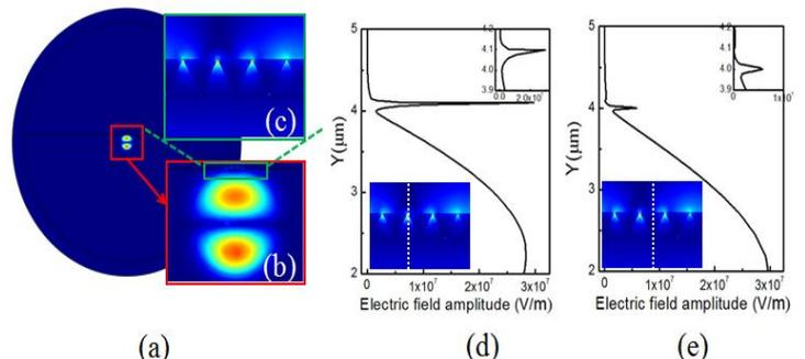
Figure 2 (a-c) Field distribution for fiber SPR sensor with RI = 1.34; Electric field density along the y-axis. When  $y = 4.1 \mu\text{m}$  (d);  $y = 4 \mu\text{m}$  (e), at the height of the gold triangle nano-rod array surface, the decay of the field is interrupted and a strong peak occurs corresponding to the plasmonic mode
