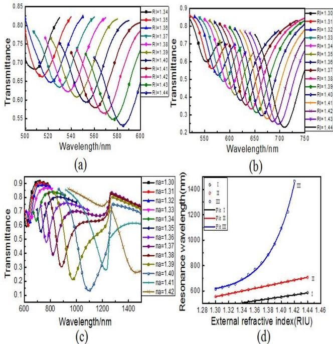
Fig.3(a-c) The wavelength shifts with the different RIU in a range of 1.30-1.43RIU; (d)The linearity of those three resonance dips.
