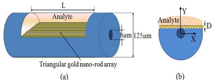
Fig.1 The 3D(a) and 2D(b) schematic of side-polished fiber optic SPR sensor based on the gold triangle nano-rod array
