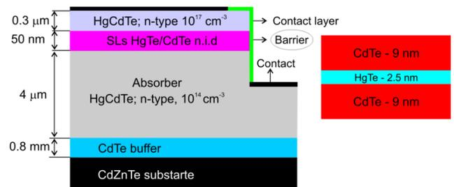
Fig. 1. Simulated nBn HgCdTe structure with HgTe/CdTe SLs barrier.
