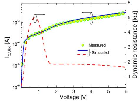
Fig. 3.  $I_{DARK}$  and  $R_D$  versus voltage for nBn detector with SLs HgTe/CdTe barrier at  $T = 155$  K.
