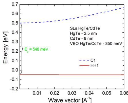
Fig. 2. Typical dispersion relation for C1 and HH1 in growth direction for HgTe/CdTe SLs at  $T = 155$  K,  $VBO = 350$  meV.
