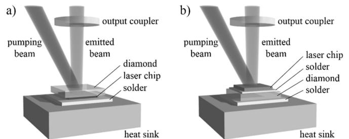
Fig. 1. Typical structure of a semiconductor disk laser with the upper (a) and bottom (b) heat spreader.
