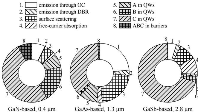
Fig. 2. Distributions of carriers generated in the active regions of the modeled lasers. OC stands for output coupler, A, B, C denote monomolecular, bimolecular and Auger recombination processes, respectively.
