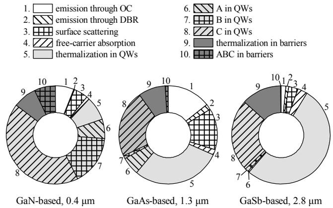
Fig. 3. Distributions of pumping power absorbed in the active regions of the modeled lasers. OC stands for output coupler, A, B, C denote monomolecular, bimolecular and Auger recombination processes, respectively.
