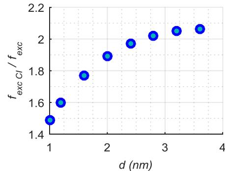
Fig. 4. Calculated dependence of ground state exciton oscillation strength on well width  $d$
