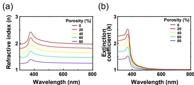
Fig. 1. (a) Calculated refractive indices (RI) and (b) extinction coefficients of ZnO with different porosities (PR) as a function of wavelength.
