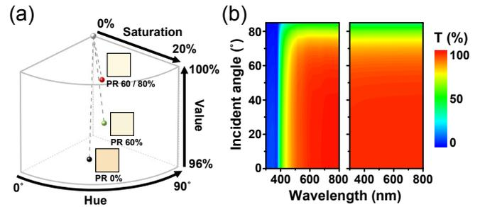
Fig. 4. (a) HSV (Hue, Saturation and Value) color coordinate containing chromatic information and color representation of PR 60 / 80%, PR 60% and PR 0%. (b) Contour maps of angle dependent transmittance of a ZnO HNS arrays with an optimized geometry (i.e., PR 60 / 80% and 300 nm layer thickness) on a glass substrate and bare glass (as a reference).
