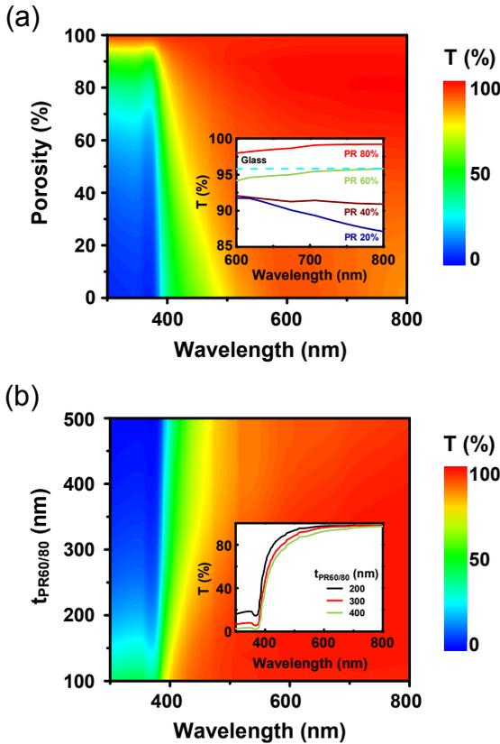
Fig. 3. (a) Contour plot of variation of transmittance of PR different ZnO thin film with a thickness of 150 nm. Inset shows enlarged transmittance spectra at 600-800 nm. (b) Contour plot of variation of transmittance of PR 60 / 80% ZnO multilayers with different thickness ( $t_{PR60/80}$ ). The thicknesses of each layer of multi-layers are equal.
