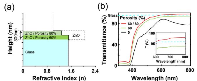
Fig. 2. (a) Refractive index profiles versus height UV absorbing transparent glass with a conventional ZnO thin film (dash line) and ZnO multilayers with different porosities (solid line). RI of each material at 500 nm were considered. (b) Transmittance spectra of glasses with the PR 0%, PR 60% ZnO thin-films and PR 60 / 80% ZnO multilayers. The thicknesses of thin films and multilayers are 300 nm.
