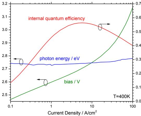
Fig. 2: Peak photon energy (blue), bias (green), and internal quantum efficiency (red) simulated at  $T=400\text{K}$ .
