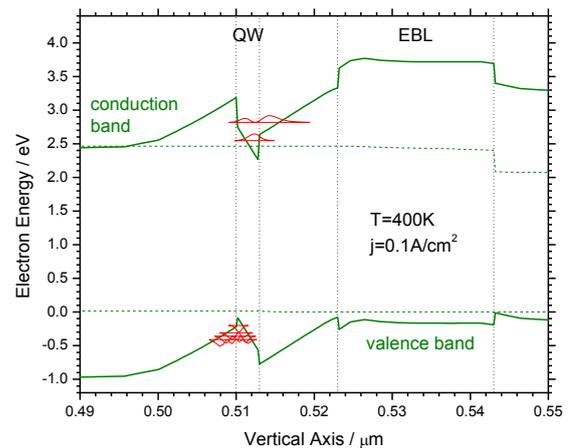
Fig. 1: Energy band diagram near the InGaIn/GaN quantum well (QW; EBL – AlGaIn electron blocking layer; dashed: quasi Fermi levels, red: quantum levels and wave functions).
