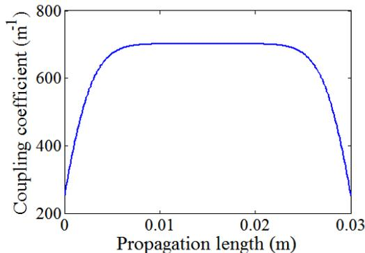
Fig. 2. Coupling coefficient variation along the length of the device due to apodization
