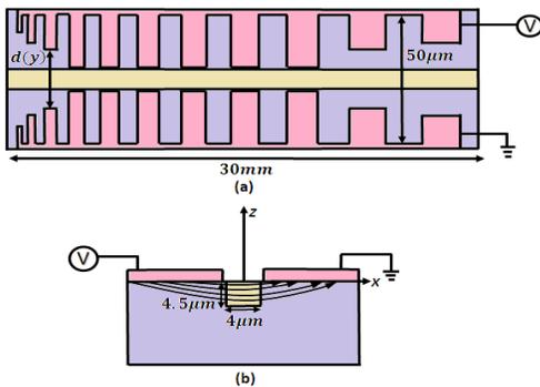
Fig. 1. Schematic diagram: (a) top view (b) cross-sectional view of z-cut LiNbO3 polarization converter.
