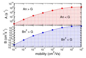
Fig. 3. Recombination parameters required such that Shockley-Read-Hall or direct/bimolecular bulk recombination becomes dominant.
