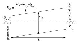
Fig. 1. Schematic bandstructure of the device model at thermodynamic equilibrium.  $E_g$  is the band gap,  $\phi_{b,a}$  and  $\phi_{b,c}$  are the Schottky barriers at the photoanode and -cathode, respectively.  $E_0$  is the electric field at equilibrium, L is the device length.
