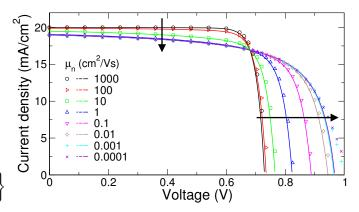
Fig. 2. Current voltage characteristics under illumination for different mobilities. The parameters are:  $N_c = 10^{19} \text{ cm}^{-3}$ ,  $E_g = 1.42 \text{ eV}$ ,  $\phi_b = 0.2 \text{ eV}$ ,  $v_s = 10^6 \text{ cm/s}$ , qGL = 20 mA, L = 100 nm. The symbols give the results of numerical drift-diffusion simulations.
