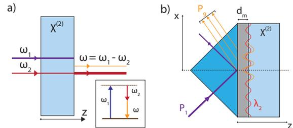
Fig. 1. a) Usual structure for DFG process. The frequency of two input beams are  $\omega_1$  and  $\omega_2$ , respectively. b) SPDC generation in Kretschmann configuration. The pump beam power is  $P_1$  and the power of generated beam is  $P_g$ .
