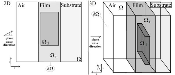
**Figure 1.** Sketch of model problem domain in 2D and 3D.  $\Omega$ ,  $\Omega_d$  and  $\Omega_T$  denotes the model, target and design domains respectively,  $\delta\Omega$  denotes the model domain boundary.
