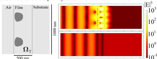
**Figure 2.** (Left) Si nanorod design in dark gray. (Right)  $|\mathbf{E}|^3$  field on  $\log_{10}$ -scale in and around the film under TM plane wave excitation at 1500 nm (top) with and (bottom) without the Si rods.
