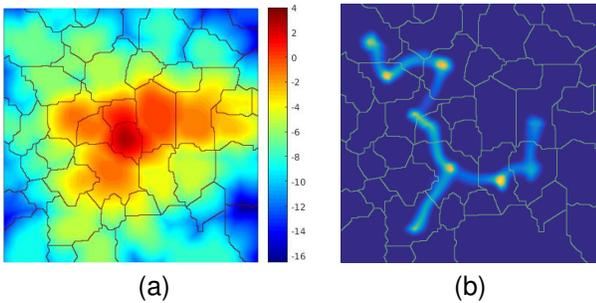
Fig. 2. (a) Agmon distance computed from the center of a localization subregion located inside the domain (log scale). (b) Examples of preferential interaction paths determined by the sum of Agmon distances (see Eq. 12). These paths essentially go through the saddles of the effective potential  $W$  displayed in Fig. 1b.
