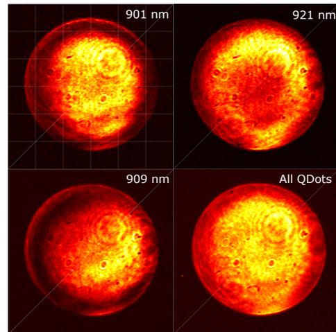
Fig. 1. Far field emission pattern of a tapered nanowire with a bottom diameter of 280 nm. Three quantum dots emitting at 901 nm, 909 nm and 921 nm are present in this sample. The far-field emission pattern are quite different indicating that the quantum dots are positioned differently in the nanowire.
