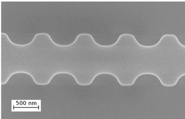
Fig. 1. SEM micrograph of analyzed silicon nitride laterally coupled waveguide Bragg grating. Single side modulation depth is 244 nm, total width 1046 nm, and grating period is 844 nm.
