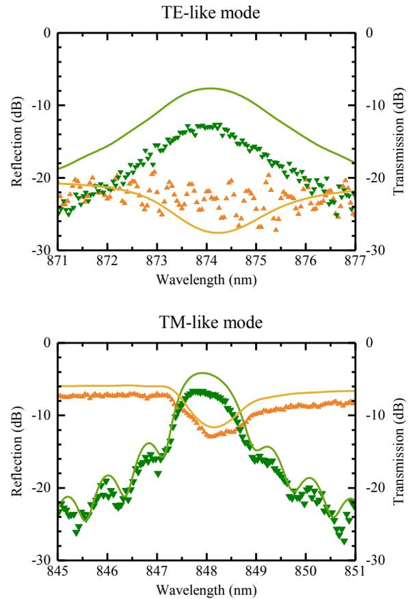
Fig. 2. Reflection and transmission spectra for TE and TM-like mode for 3<sup>rd</sup> order laterally coupled Bragg grating. Dimensions for CWT simulations are calculated from SEM micrograph. (▲ trans. measured, ▼ refl. measured, — trans. CWT, — refl. CWT)
