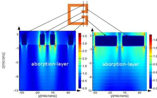
Fig. 3. The sectional view of electromagnetic field distribution at the split of the ring and the absorption-layer below.
