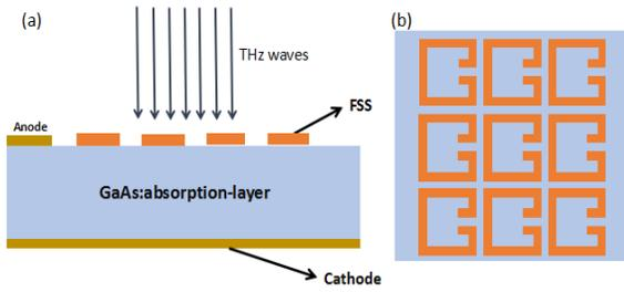
Fig. 1. Diagram of the GaAs device with periodic split-ring-shaped array.
