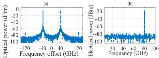
Fig. 1. (a) Optical spectrum and (b) electrical spectrum of the frequency 8-tupling signal
