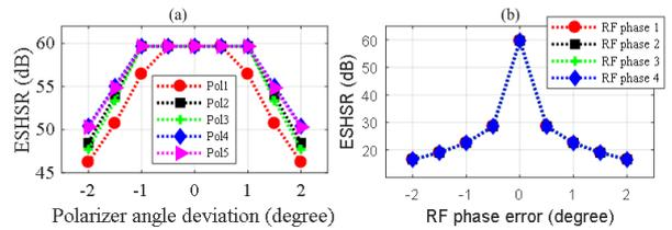
Fig. 4. ESHSR variation due to the drift of (a) polarizer angle and (b) RF drive phase from ideal condition
