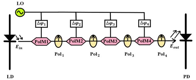
Fig. 1. Schematic diagram of the proposed frequency octupling architecture. LD: laser diode; PD: photo-diode; LO: local oscillator.
