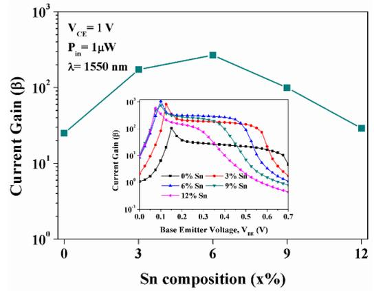
Figure 3 Current gain variation with different Sn concentration in base for a fixed emitter and sub-collector doping. Inset shows the Current gain variation with applied base emitter voltage for different Sn concentration in base for a fixed emitter and sub-collector doping.
