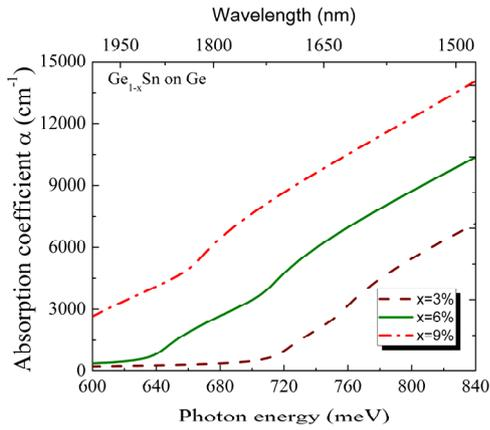
Figure 2 Absorption coefficient for pseudomorphic GeSn on Ge substrate
