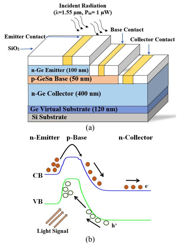
Figure 1(a) Schematic of the n-p-n HPT (b) Simulated band diagram of device structure
