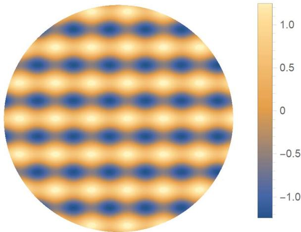
Fig. 1 Electric field in the static magnetic field area. There are just two propagation directions, the incident direction is the  $y$  direction. The exchange factor in this calculation is 0.3.
