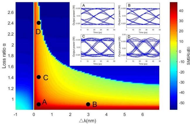
Fig. 2 SMSR for different wavelength interval and loss ratio. Insert : eye diagrams for four cases: 1) case A,  $\Delta\lambda=0.28\text{nm}$ ,  $\alpha=0.9$ , SMSR=38.34dB; 2) case B,  $\Delta\lambda=3\text{nm}$ ,  $\alpha=0.9$ , SMSR=22.19dB; case C,  $\Delta\lambda=0.28\text{nm}$ ,  $\alpha=1.4$ , SMSR=21.77dB; 4) case D,  $\Delta\lambda=0.28\text{nm}$ ,  $\alpha=2.4$ , SMSR=15.83dB
