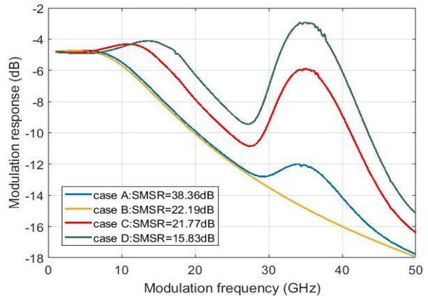
Fig. 3. Small signal response for different cases
