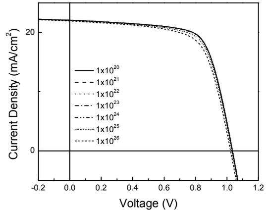
Fig. 3. Simulated J-V curves for different effective hole trap densities.
