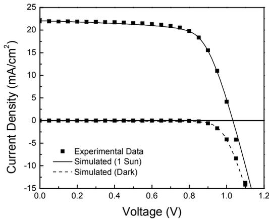
Fig. 1. Simulated J-V curve under 1 sun illumination and in the dark compared with experimental data obtained.
