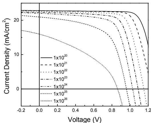
Fig. 2. Simulated J-V curves for different effective electron trap densities.
