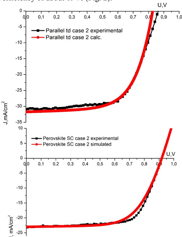
Fig. 2 Simulated and experimental dependences with connecting in-parallel and in-series
