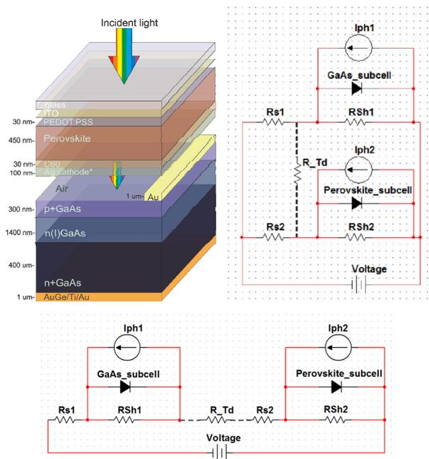
Fig. 1 Tandem device schematics (GaAs- perovskite tandem at short circuit regime); equivalent circuits of parallel and in-series tandems for single diode simulation
