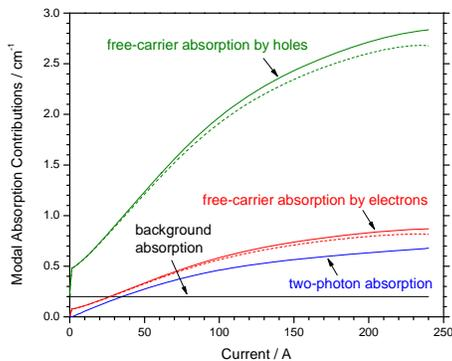
Fig. 2: Contributions of the different absorption mechanisms to the modal optical loss vs. current. Solid lines: full model. Dashed lines: free-carrier absorption without two-photon absorption.
