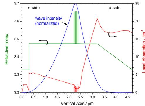
Fig. 1: Vertical profiles of refractive index, wave intensity (normalized), and local absorption.
