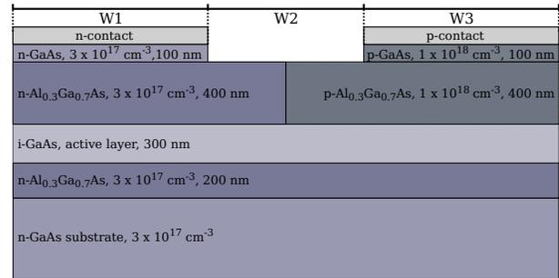
Fig. 1. Schematic structure of one period of the studied LHJ GaAs/AlGaAs DDCT LED.
