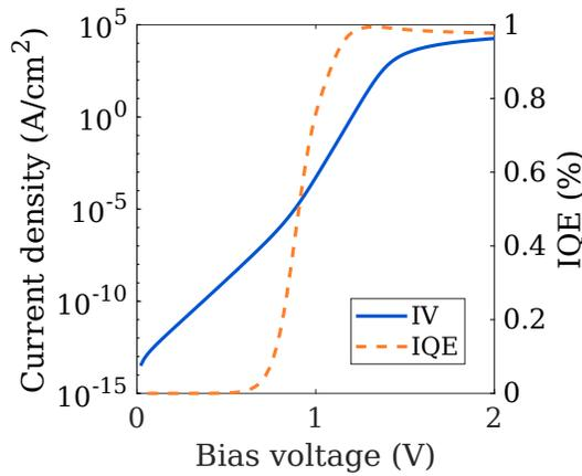
Fig. 2. The  $I-V$  curve showing SRH and radiative recombination dominated regimes. The IQE of the device starts to increase as radiative recombination starts to dominate, and stays over 97 % at biases above 1.2 V.
