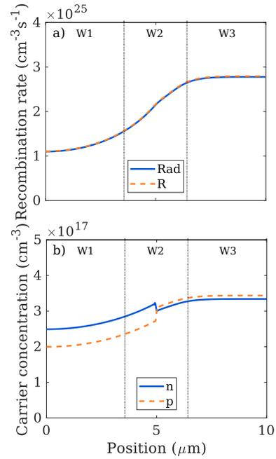
Fig. 3. (a) Radiative and total recombination rates and (b) the carrier concentrations within the AL as a function of lateral position at  $J = 100 \text{ A/cm}^2$ .
