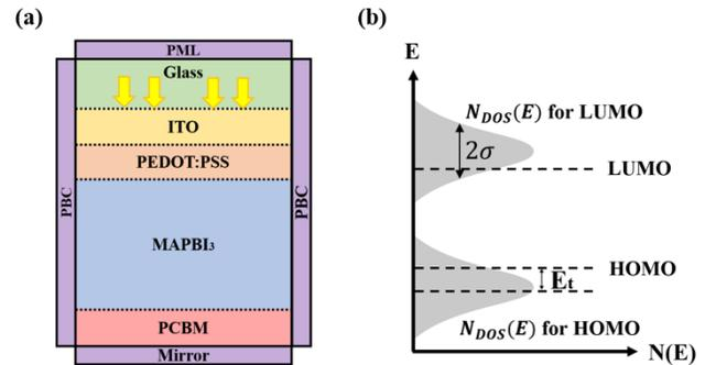
Fig. 1. (a) The simulated structure with 2D-FDTD optical solver; (b) The Gaussian-like density of states.
