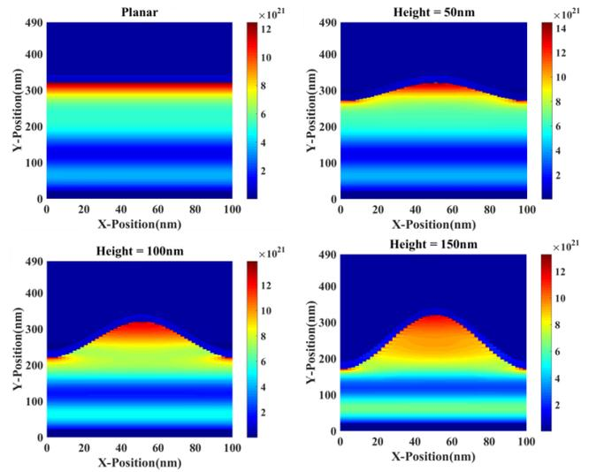
Fig. 3. The generation rate of the solar cells with different height of curvature.
