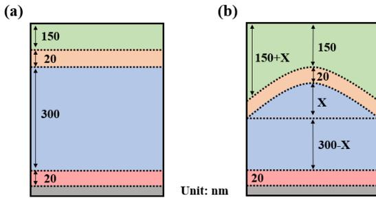
Fig. 2. (a) The structure of planar perovskite solar cells; (b) The structure of nano-structure perovskite solar cells, where X is the height of curvature.
