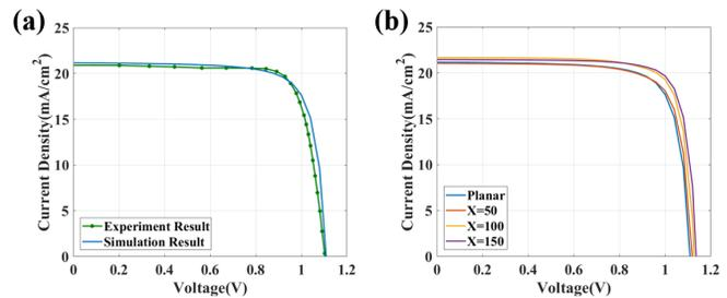
Fig. 4. (a) The  $J$ - $V$  curves of the planar solar cells; (b) The  $J$ - $V$  curves of the nano-structure solar cells.
