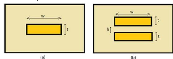
Fig. 1. Waveguide cross section of (a) SS, (b) DS configuration.
