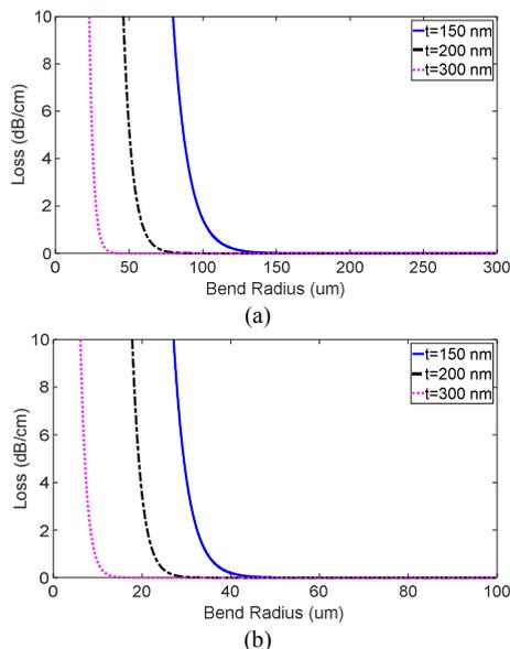
Fig. 2. Bend loss versus bend radius at 1550 nm for (a) SS, (b) DS waveguides with  $h=50$  nm
