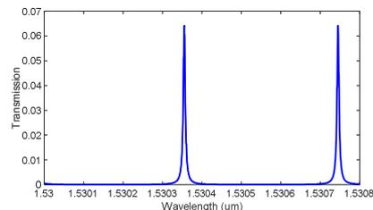
Fig. 4. Power transmission of add-drop single ring filter of 650  $\mu\text{m}$  radius
