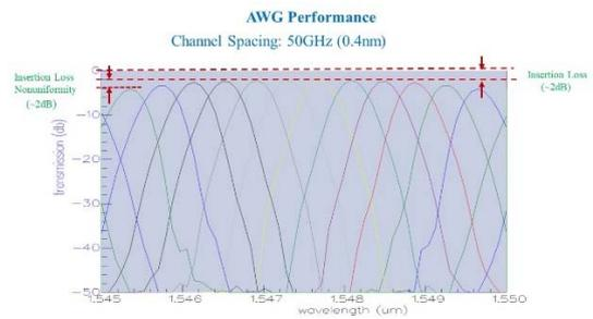
Fig. 3. Transmission spectrum of AWG.
