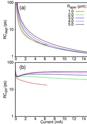
Fig. 3. RC-product for the depletion (a) and diffusion (b) capacitance of the VCSEL versus current for the aperture thickness  $20 \text{ nm}$  and different aperture radii.
