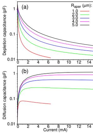
Fig. 2. Depletion (a) and diffusion (b) capacitance of the VCSEL versus current for the aperture thickness  $20 \text{ nm}$  and different aperture radii.
