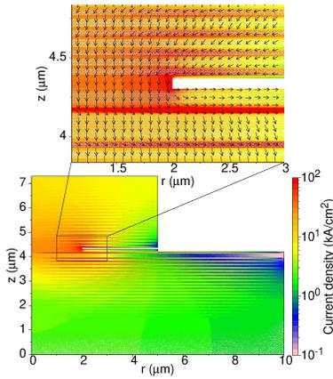
Fig. 1. Spatial distribution of the current density magnitude in the color map view for the aperture radius  $2 \mu\text{m}$ , thickness  $70 \text{ nm}$  and circular n- and p-contacts at the bottom of the substrate and at the top of the VCSEL mesa, respectively, at the bias  $2 \text{ V}$  and the current  $5.3 \text{ mA}$ . The upper panel shows also the current flow directions in the vicinity of the aperture and active region.
