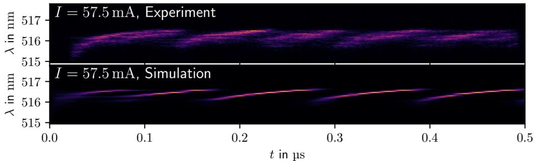
Fig. 1. Measured and simulated streak camera images for a green nitride laser diode with a cavity length of 900  $\mu\text{m}$ . Here the laser output is shown as function of time and wavelength. The simulation uses an effective coupling term as given in Eq. (1).
