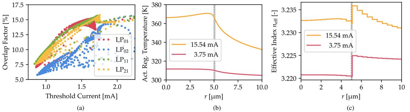
Fig. 2. The correlation between the overlap factor and the threshold current (a), temperature profile (b) and effective index distribution (c) in the active region for input currents of 3.75 mA and 15.54 mA.
