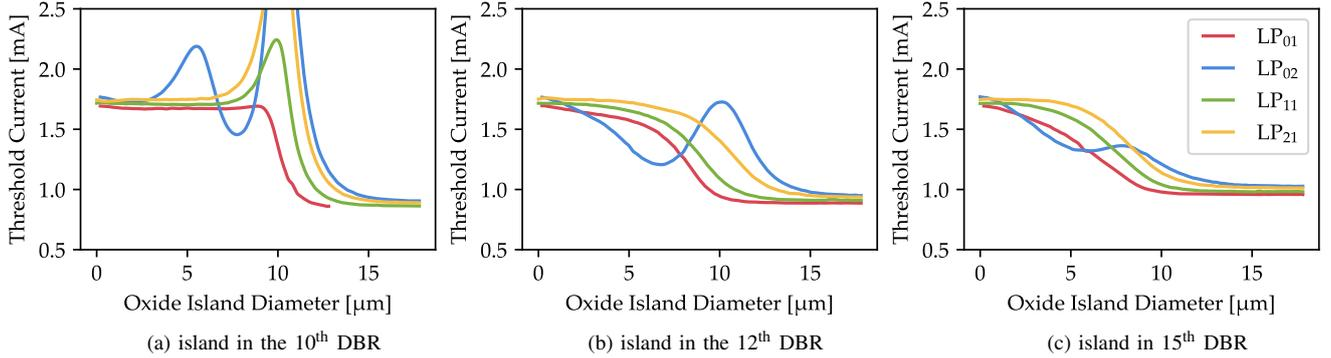
Fig. 1. Dependence of threshold current on the size of the oxide island for several locations in the DBR layers. The position of the island has a strong impact the qualitative behavior of the modes. Below the 12<sup>th</sup> pair, strong oscillations are visible. A rapid increase in threshold current can be observed for critical island diameters (10  $\mu\text{m}$  and around 5  $\mu\text{m}$  for the LP<sub>02</sub> mode).
