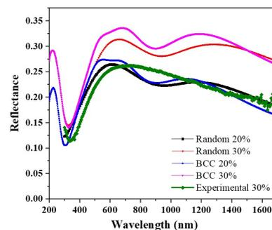
Fig. 1. Comparison of FDTD (*bcc* and random particle distribution) and experimental reflectance. FDTD used bulk Mo optical parameters and metal volume fraction  $f=20\%$  and  $30\%$ .
