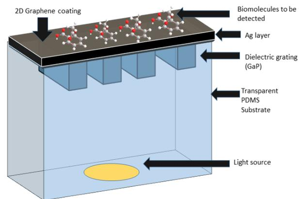
Figure 1: Structure of the biosensor.
