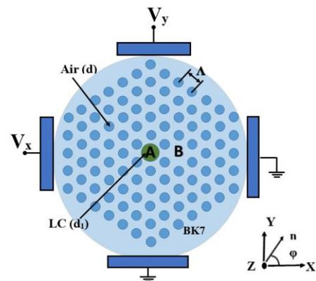
Fig. 1. Cross section of the proposed ADC-PCF.
