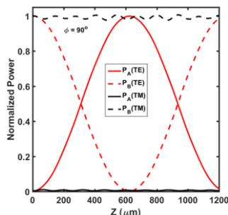
Fig. 3 Normalized powers for both polarizations in cores A and B at  $\phi=90^\circ$  at  $\lambda=1.3\ \mu\text{m}$ .
