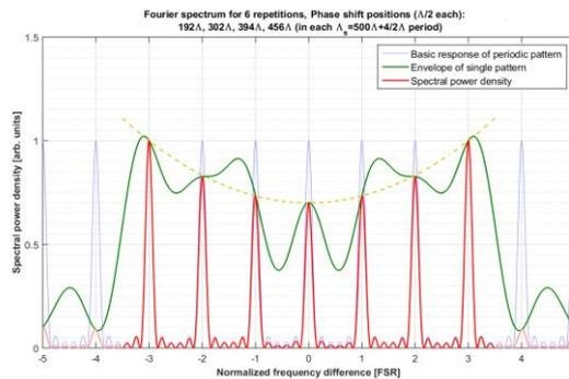
Fig. 3. 7-peaked phase-modulated grating design with curved envelope
