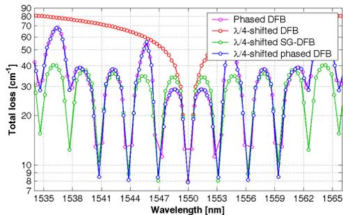
Fig. 1. Loss versus wavelength comparison of various DFB laser cavities
