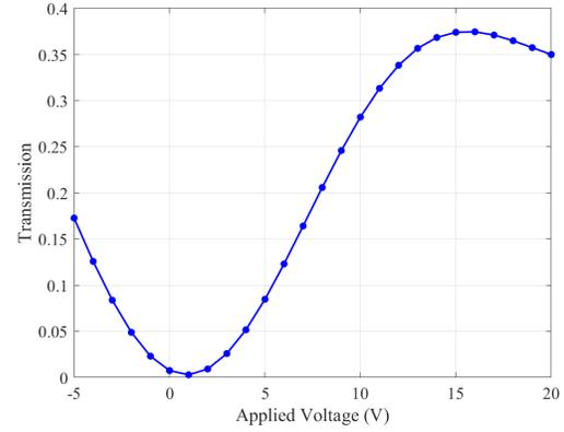
Fig. 4. Modulator DC transmission versus applied voltage.
