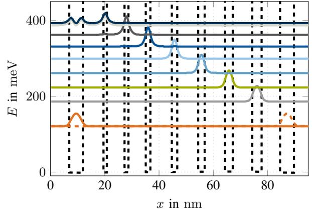
Fig. 1. Calculated conduction band profile and probability densities of the investigated mid-IR QCD structure N1022 [12] detecting at  $4.7\ \mu\text{m}$ . Space charge effects are included by solving self-consistently the Schrödinger and Poisson equation. The electron densities in each state are modeled accounting for thermal equilibrium under zero external bias and no incident light.
