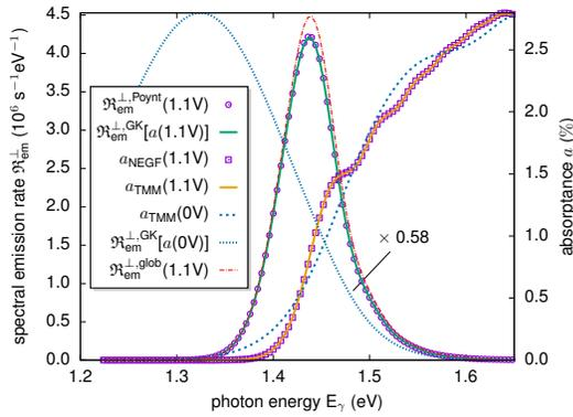
Fig. 2. Absorptance and front-side emission of a 100 nm GaAs p-i-n solar cell with gold rear reflector, reflecting the impacts of built-in field variation and reabsorption [7].
