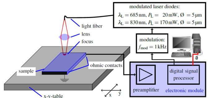
Fig. 2. LPS measurement setup.
