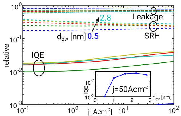
Fig. 2. IQE as well as relative contribution of the leakage current and Shockley-Read-Hall recombination to the total LED current. The inset shows the variation of the IQE with the QW width at  $j = 50 \text{ Acm}^{-2}$ .
