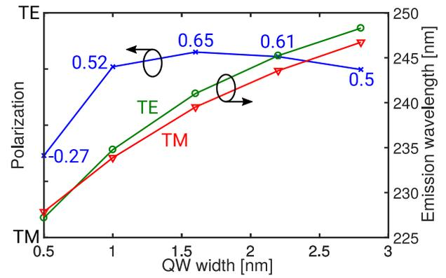
Fig. 1. Simulated light polarization and emission wavelength versus QW width at  $j = 50 \text{ Acm}^{-2}$ . Only the 0.5nm QW shows dominant TM-polarization. Wider QWs show generally dominant TE-polarization.
