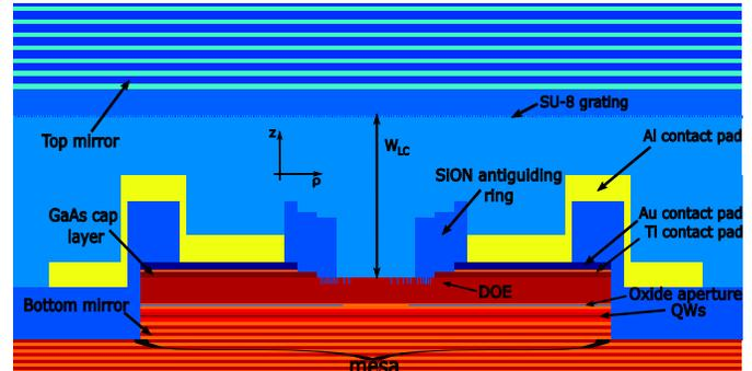
Fig. 1: Sketch of the top-emitting tunable VCSEL highlighting the relevant parts: the mesa, the LC cavity  $w_{LC}$ , the QWs, the top (output) and bottom DBRs, the electrode pad to inject current in the active material, the alignment grating, the DOE and the antiguiding structure for mode selection. The color map indicates refractive index values from low (blue) to high (red).
