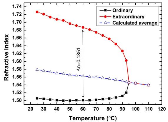
Fig. 3: Refractive indices measured at 1.55  $\mu\text{m}$  for extraordinary (red) and ordinary (black) polarizations as a function of temperature for a QYDPLC-036-based filter. The average index is plotted in blue.
