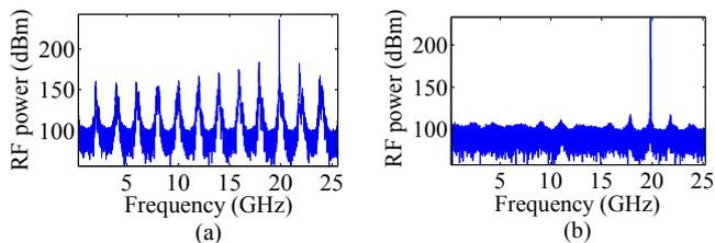
Fig. 3. Electrical spectrum (RBW=1 MHz) of tenth harmonic of without-intracavity (a) and with-intracavity long ring laser (b).
