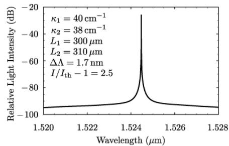
Fig.5 Oscillation spectrum.
