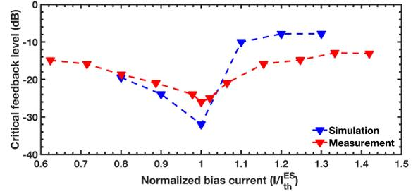
Fig. 4. Critical feedback level ( $r_{crit}$ ) as a function of the ratio of the bias current normalized to the ES lasing threshold ( $I/I_{th}^{ES}$ ) for simulation (blue) and measurement (red). Measurement is reproduced from [3].
