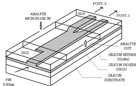
Fig. 1. The layout of biosensor based on  $\text{Si}_3\text{N}_4$  rib-optical waveguides.
