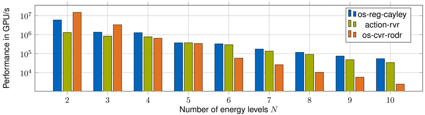
Fig. 1. Single-thread performance of the three methods that solve the Lindblad equation numerically. The metric grid point updates per second (GPU/s) is used as figure of merit. It is calculated as  $P = N_x N_t / t_{\text{exec}}$ , where  $N_x$ ,  $N_t$  denote the number of spatial and temporal grid points, respectively, and  $t_{\text{exec}}$  is the measured execution time.
