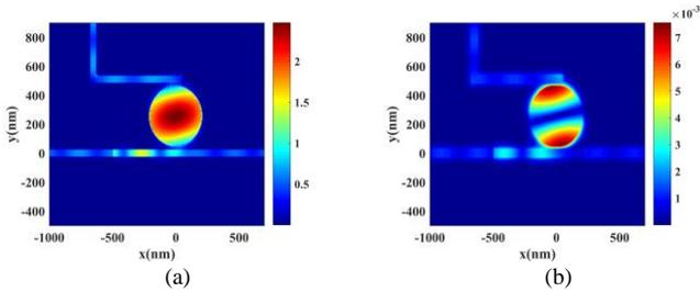
Fig. 2. (a) Electric and (b) Magnetic field intensity distributions of the 1-channel structure at resonance wavelength of  $\lambda=840$ nm.
