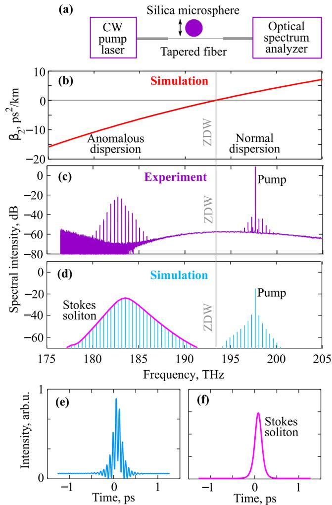
Fig. 1. (a). A simplified experimental scheme. Numerically calculated dispersion for a silica microsphere with a diameter of  $165 \mu\text{m}$ . (c) The experimental spectrum demonstrating Stokes soliton-like OFC and (d) the corresponding numerically simulated spectrum. (e) Numerically simulated intensity distribution in the time domain. (f) Numerically simulated intensity distribution of the filtered out Stokes soliton in the time domain.
