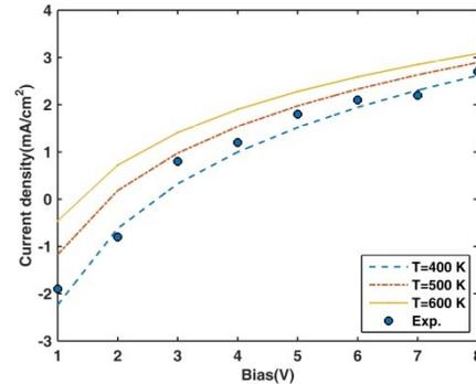
Fig. 3. Current density for varying bias at different temperatures in presence of traps
