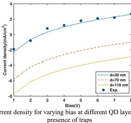
Fig. 2. Current density for varying bias at different QD layer thickness in presence of traps
