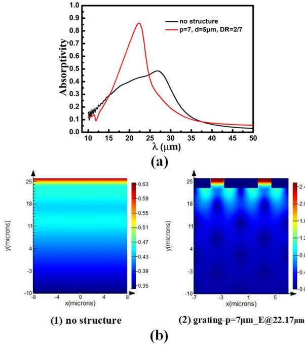
Fig.2. The absorption properties of the Si-based BIB device with metal gratings (parameters:  $p=7\mu\text{m}$ ,  $d=5\mu\text{m}$ ,  $DR=2/7$ ) compared with that of device without metal gratings. (a) The absorption spectrum; (b) The longitudinal profile of of electric field intensity.
